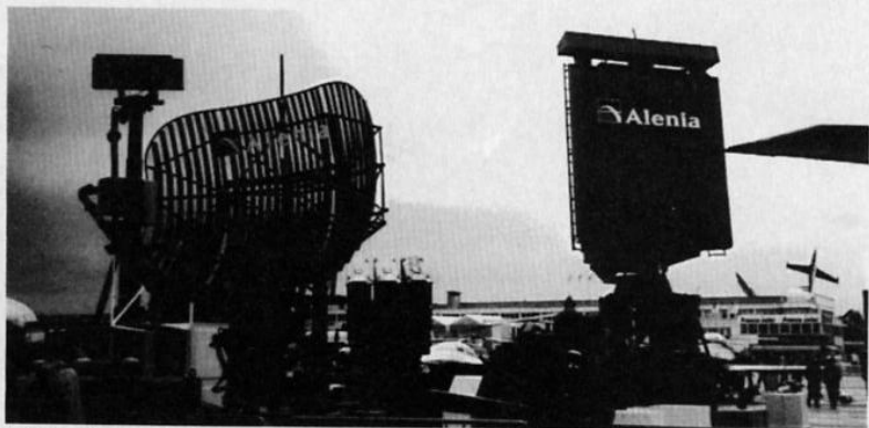
Italy's Alenia displays its newest tactical radar systems, including the RAT-31 S, three-dimensional range surveillance radar (right).
