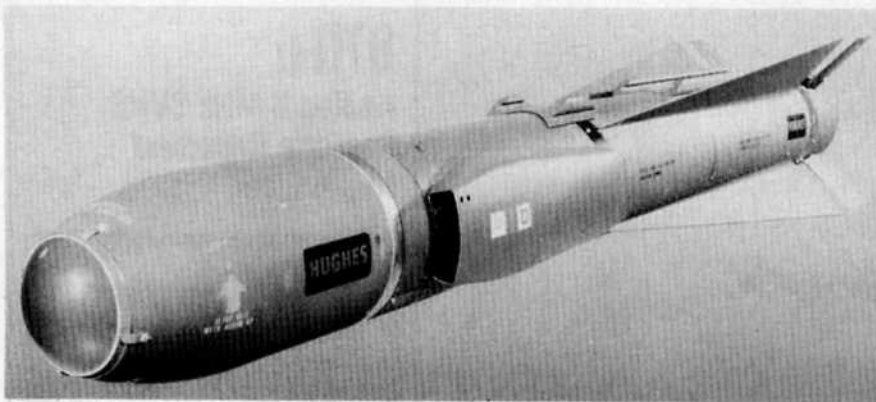
The Hughes Longhorn missile, a variant of the Maverick, is propelled by a turbine engine and has a range of 40 nautical miles. Note the infrared seeker on the missile's nose. A millimeter wave radar version is under development.
