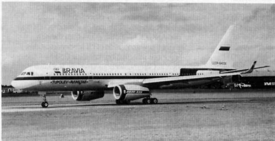
Russia's Tupolev Tu-204 passenger airliner has the United Kingdom's Rolls-Royce 535E4 engines.
